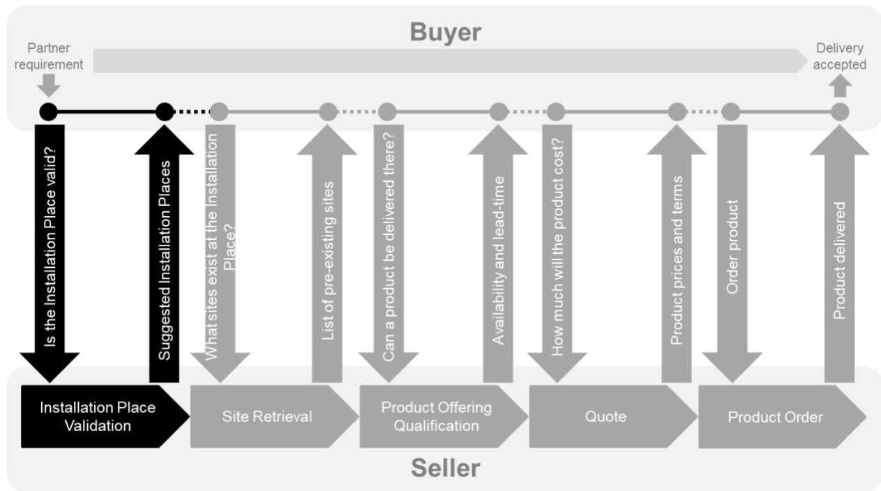
Figure 2 – Cantata/Sonata Interface Installation Place Validation
